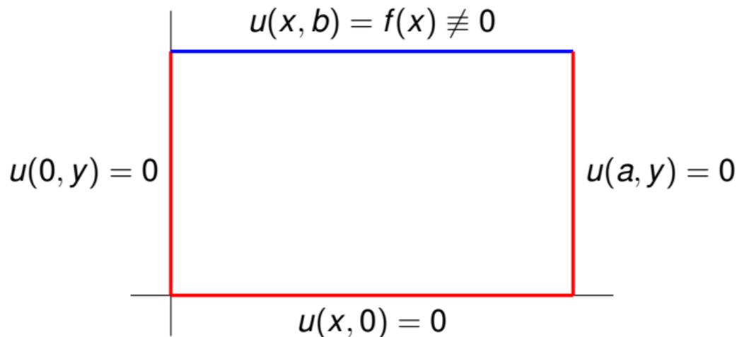
$$u(x, y) = \sum_{n=1}^{\infty} c_n \sin\left(\frac{n\pi}{a}x\right) \sinh\left(\frac{n\pi}{a}y\right) \quad \text{mit} \quad c_n = \frac{2}{a \sinh\left(\frac{n\pi}{a}b\right)} \int_0^a f(x) \sin\left(\frac{n\pi}{a}x\right) dx.$$
