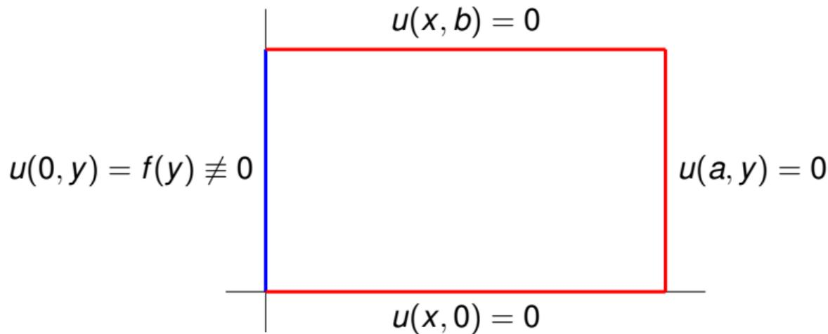
$$u(x, y) = \sum_{n=1}^{\infty} c_n \sinh\left(\frac{n\pi}{b}(x-a)\right) \sin\left(\frac{n\pi}{b}y\right) \quad \text{mit} \quad c_n = \frac{-2}{b \sinh\left(\frac{n\pi}{b}a\right)} \int_0^b f(y) \sin\left(\frac{n\pi}{b}y\right) dy.$$
