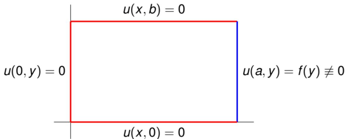
$$u(x, y) = \sum_{n=1}^{\infty} c_n \sinh\left(\frac{n\pi}{b}x\right) \sin\left(\frac{n\pi}{b}y\right) \quad \text{mit} \quad c_n = \frac{2}{b \sinh\left(\frac{n\pi}{b}a\right)} \int_0^b f(y) \sin\left(\frac{n\pi}{b}y\right) dy.$$
