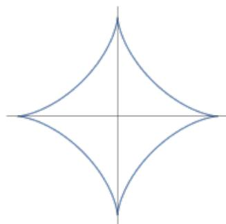
$$\begin{aligned} x(t) &= a \cos^3 t \\ y(t) &= a \sin^3 t, \quad \text{für } 0 \leq t \leq 2\pi. \end{aligned}$$
