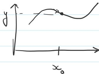
• Prop  $\lim_{\substack{x \rightarrow x_0 \\ x \neq x_0}} f(x) = y \iff \forall (x_k)_{k \in \mathbb{N}} \in X \rightarrow x_0 : (f(x_k))_k \rightarrow y$
