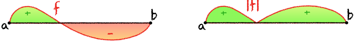
Figure 6.4: The graph of a function f is shown on the left, the graph of the corresponding function |f| is shown on the right. The integral \int_a^b f \, dx describes a net area and \int_a^b |f| \, dx a gross area.
